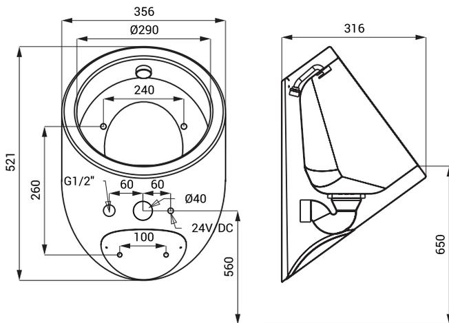
\* for the height of the front edge of the urinal 650 mm above the floor
