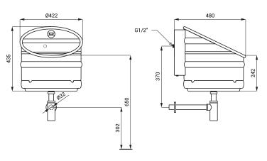
\* for the height of the front edge of the urinal 650 mm above the floor
