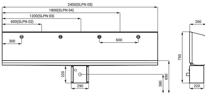
\* for the height of the front edge of the urinal 650 mm above the floor
