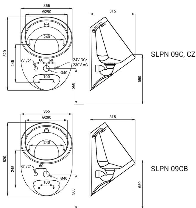
\* for the height of the front edge of the urinal 650 mm above the floor
